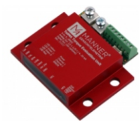
OEM Version Ip40 Dimensions: 60,0 mm x 51 mm x 15,491 mm
