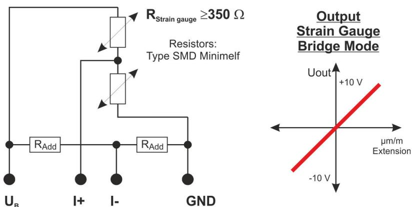
Fig. 7: Operation mode strain gauge (half bridge)
