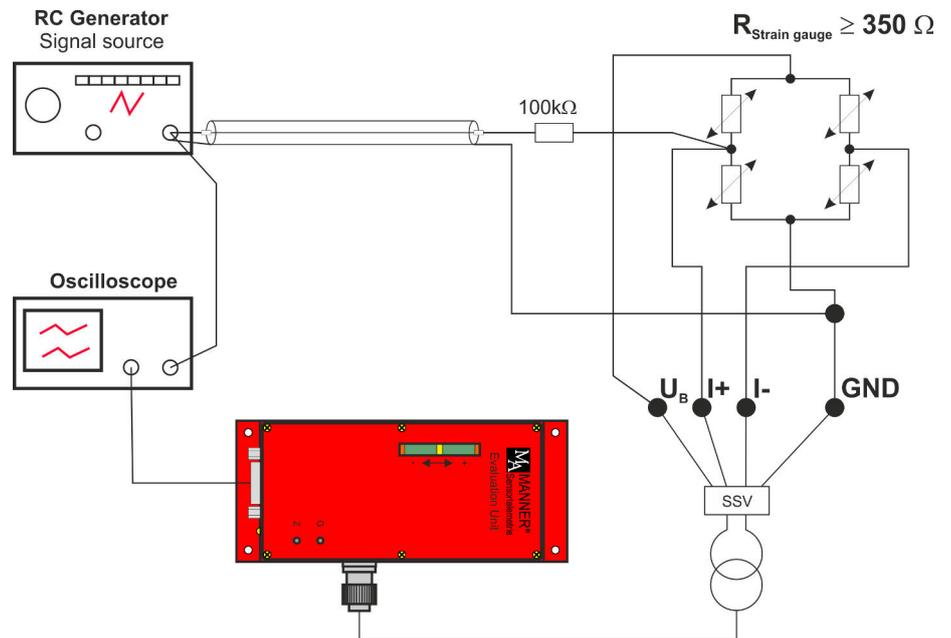
Fig. 14: Test circuit
