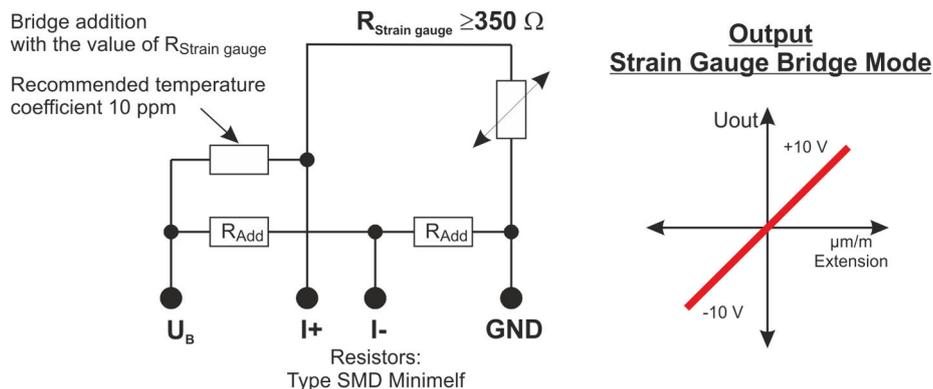
Fig. 8: Operation mode strain gauge (quarter bridge)
