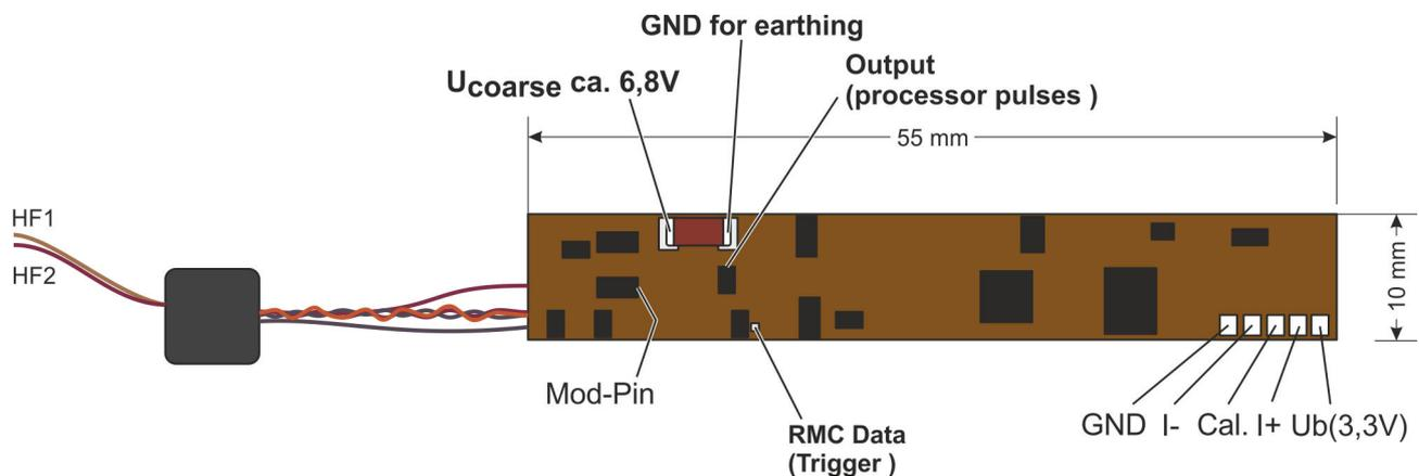
Fig. 4: SV\_flex\_PCM16\_RMC, Pin assignment
