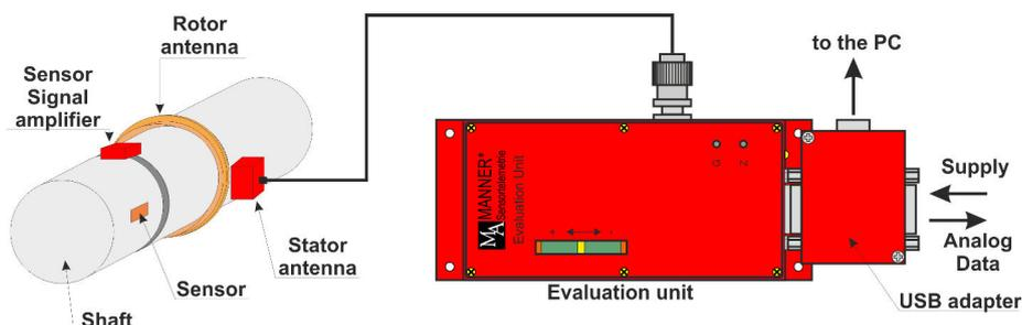
Fig. 1: General measuring configuration
