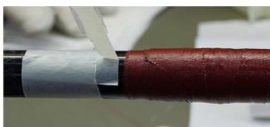
**14.**▶ Remove the masking tape with the sealing is wet.
