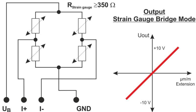
Fig. 6: Operation mode strain gauge (full bridge)
