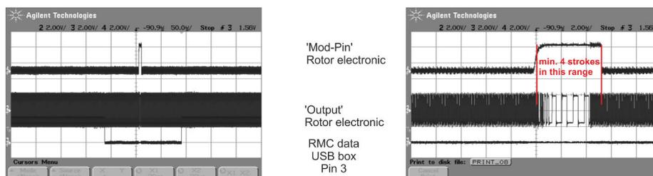
5. ▶ Alternative this function can be tested without oscilloscope by checking the screen display of the function 'Test Connection' during the Variation of the antenna distance (the acknowledge display must be shown in black; red signals a failure). With this method however the security stock can not be estimated.
